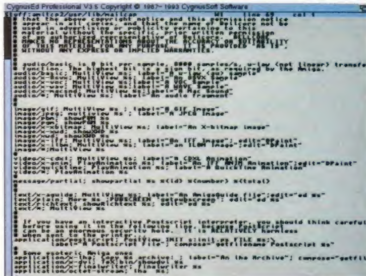
The Mailcap file contains the information needed to translate incoming MIME messages back into their original format.
